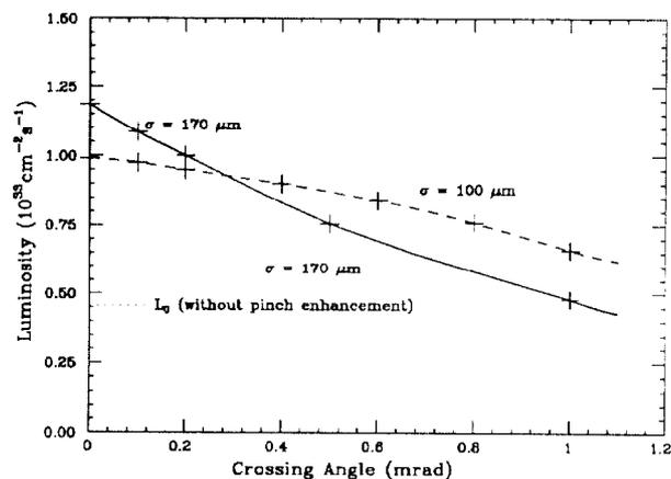
Fig.1: Luminosity dependence on crossing angle
