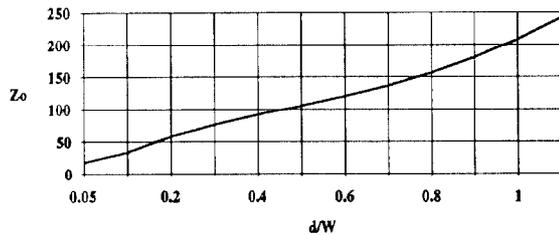
Fig. 3 - Characteristic impedance as a function of plate dimensions.
