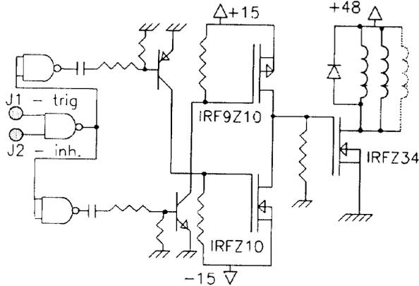
Fig. 5 - Simplified schematic of excitation circuit
