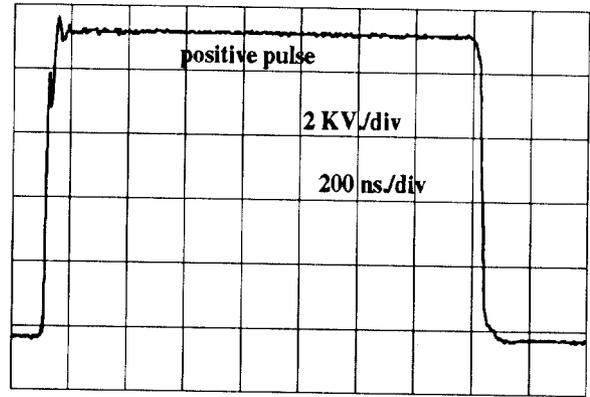
Fig. 6- Scope trace of the full positive driving pulse.
