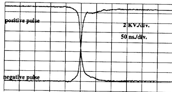
Fig. 7 - Detail of the fall time waveform for both kicker driving pulses.
