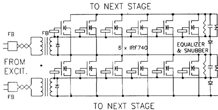
Fig. 4 - Kicker driver power section schematic (2 of 26 sections shown).
