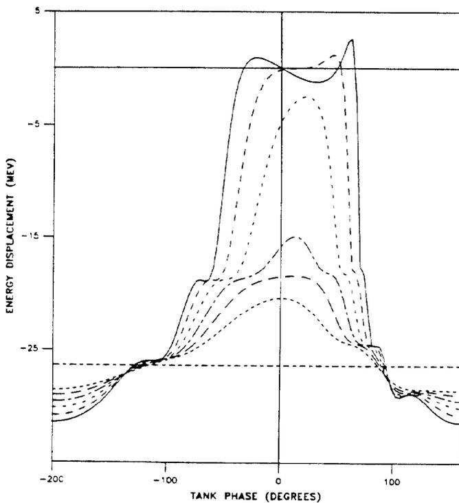
Figure 1. Energy displacement versus tank phase for tank number 4 of the existing Fermilab Linac.
