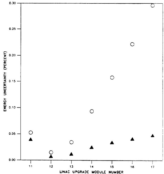
Figure 2. Output energy uncertainty for 13.8 picosecond random error in time measurement. Circles - Method # 1 triangles - Method # 2. The two methods are described in Section III.
