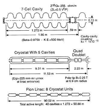
Figure 4. Reference linac configuration.
