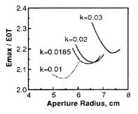
Figure 1. Peak surface field per unit accelerating gradient for cavities with circular noses for several values of cell-to-cell coupling parameter k.
