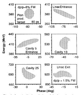
Fig. 6. Longitudinal evolution of the beam bunch.
