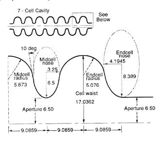
Figure 2. Pilac cavity geometry. All dimensions are in cm.
