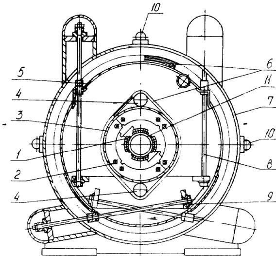
Fig. 5. Cross sectional view of a SC quad assembled in a force-circulating cryostat: 1 - coil, 2 - magnet shield, 3 - helium vessel, 4 - two-phase helium pipe, 5 - thermal shield, 6 - superinsulation, 7 - vacuum shell, 8 - suspension, 9 - extension rod, 10 - geodetic marks, 11 - ion pipe.
