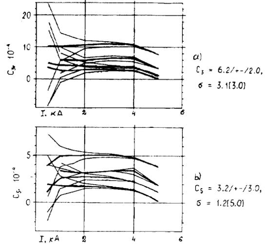
Fig. 9. Bore field nonlinearities of 4 SC dipoles at a radius of 3.5 cm versus the coil current.
