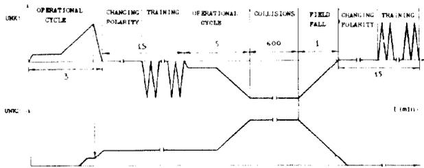
Fig. 2. Operational scheme of the 0.4x3 TeV UNK collider.
