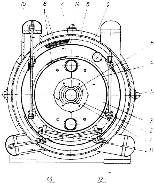
Fig. 4. Cross sectional view of a SC dipole assembled in a force-circulating cryostat: 1 - coil, 2 - collars, 3 - magnetic shield, 4 - helium vessel, 5 - two-phase helium pipe, 6 - ion pipe, 7 - thermal shield, 8 - superinsulation, 9 - vacuum vessel, 10 - suspension, 11 - extension rod, 12 - single-phase helium, 13 - two-phase helium, 14 - geodetic marks.
