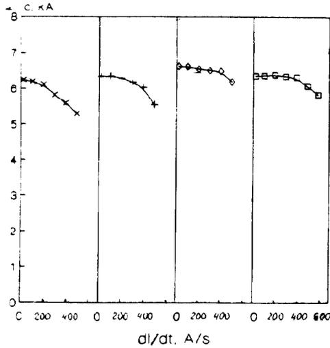
Fig. 7. Ramp rate characteristics of SC dipoles: o - DDXB2, □ - DDXB4, △ - DDXB6.
