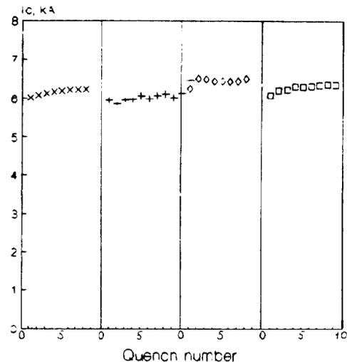
Fig. 6. Training curves for SC dipoles: <- DDXB1, o - DDXB2, Δ - DDXB6.
