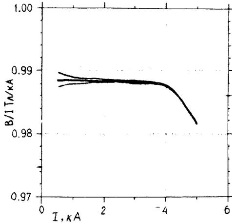
Fig. 8. Transfer function of a SC dipole versus the coil current.
