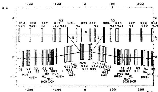
Fig. 3. Optical scheme of Matched Straight Section 6 for colliding beams.
