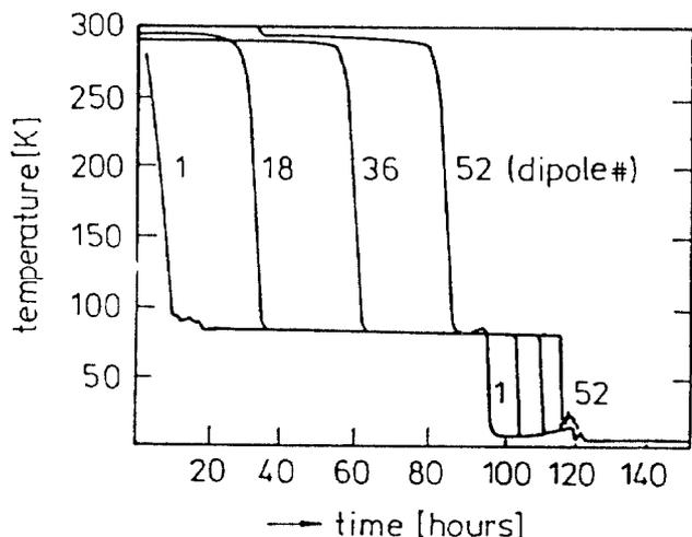
Fig. 3 - Cooldown profile of a HERA octant.
