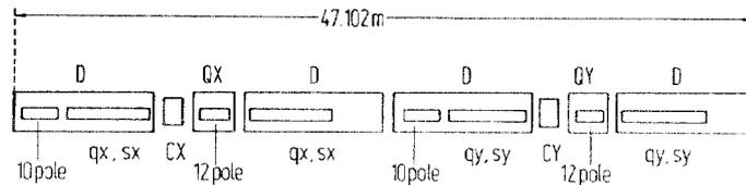
Fig. 5 - A unit cell of the proton ring. D: main dipole; QX, QY: main quadrupoles, qx, qy: quadrupole correction coils, sx, sy: sextupole correction coils, CX, CY: correction dipoles. In addition, there are 10-pole and 12-pole correction coils.
