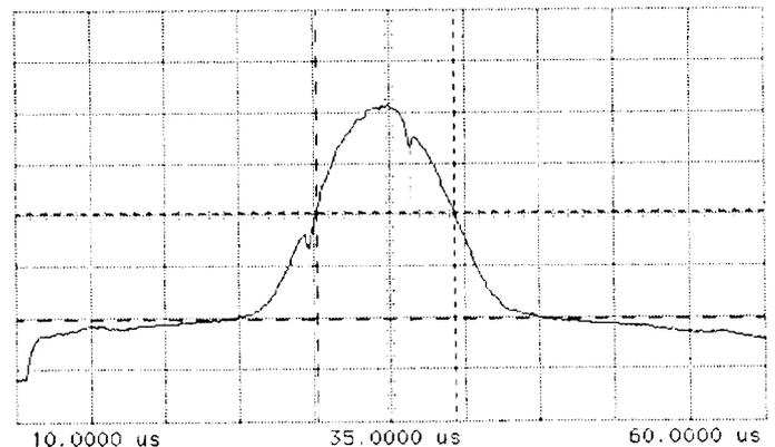
Fig. 7 - Beam profile measured with the residual gas monitor. Full width at half height is 13.8 mm.
