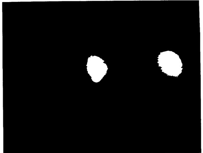
Fig. 6 - Images of the injected beam (right spot) and of 5 successive turns (left spot) on a screen close to the septum magnet. The distance between the spots is 3 cm.
