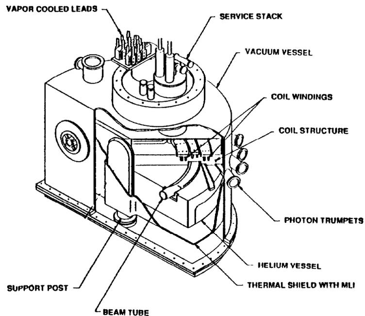
Figure 3. A superconducting dipole magnet assembly
