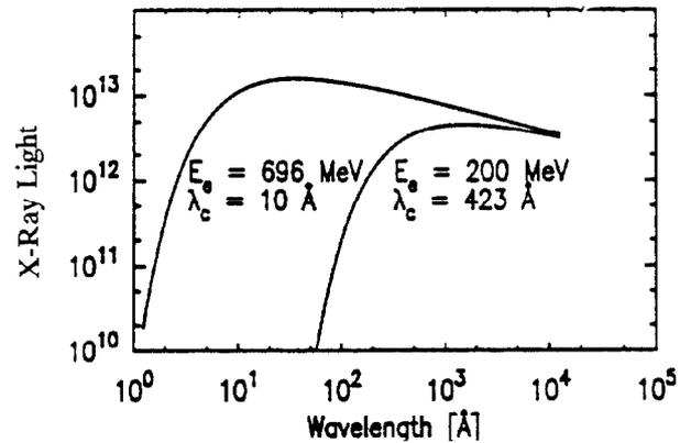
Figure 4. Synchrotron radiation as a function of wavelength
