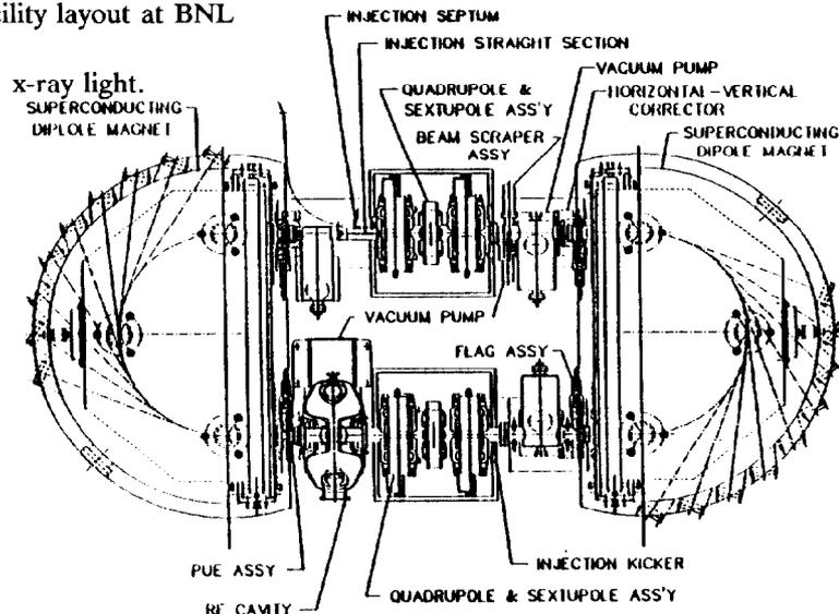
Figure 2. Plan view of the SXLS ring
