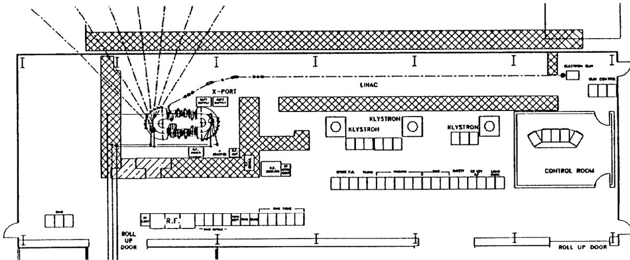
Figure 1. SXLS Facility layout at BNL
