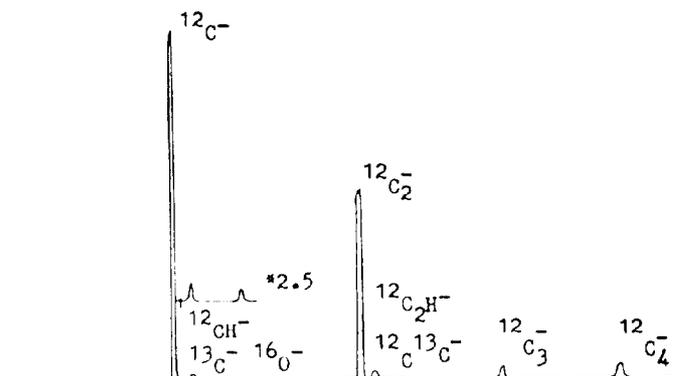
Fig. 2. Spectrum of the new sputter ion source with a graphite target on AMS injector
