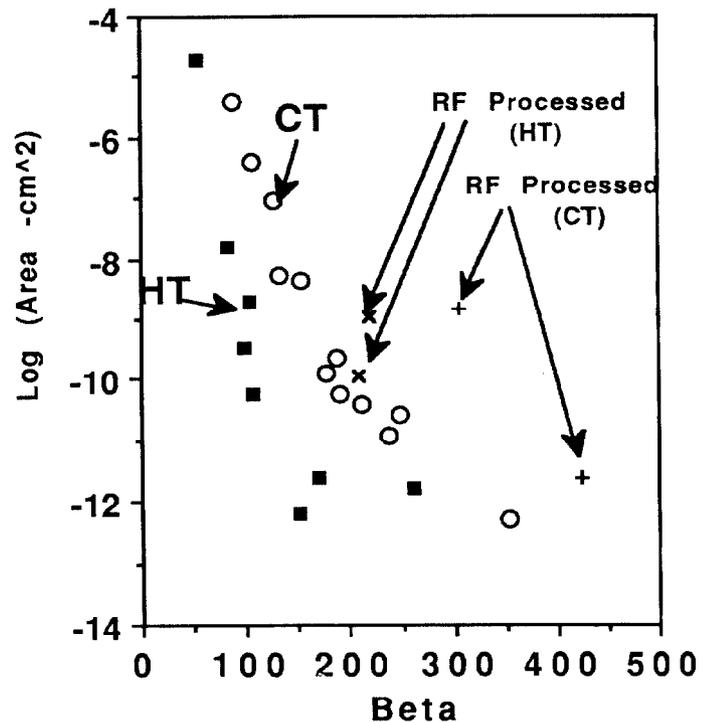
Fig. 4: Fowler Nordheim properties of emitters found in chemically treated (CT) and heat treated (HT) cavities
