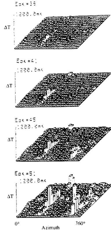
Fig. 3: Appearance of field emitters in a heat treated cavity as the field level is raised from  $E_{pk} = 36$  to  $51$  MV/m
