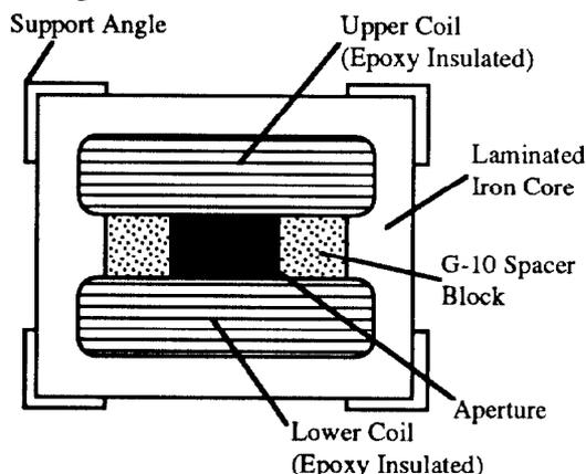
Figure 1. Schematic end view of 200 turn dipole.
