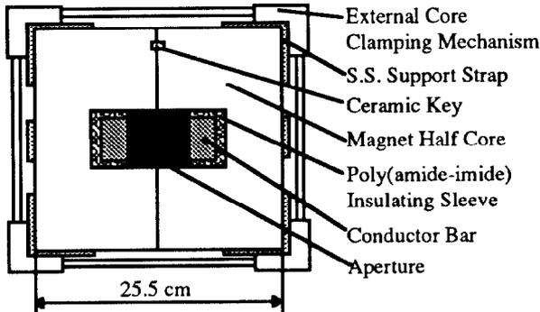
Figure 2. Schematic cross section view of Single Turn dipole (water cooling and coil tie rod details omitted for clarity)
