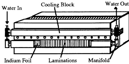
Figure 4. Schematic view of water cooling system (some details omitted for clarity).
