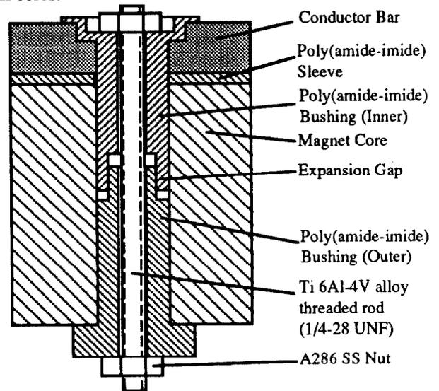
Figure 3. Cross section view of typical coil to core assembly
