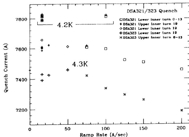
Fig.4: Ramp Rate Dependence of Quench Current
