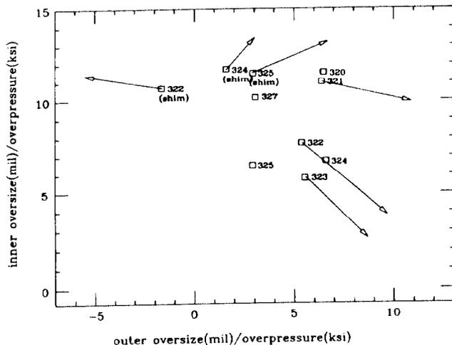
Fig.2: Size-Pressure Plot. Marked positions with magnet number represent the oversize of both coils in that magnet. The arrow represent the vector  $(p_i - p_i^d, p_o - p_o^d)$ , where  $p_i$  and  $p_o$  are the inner and outer coil pressure. Suffiz <sup>d</sup> refers to design values.
