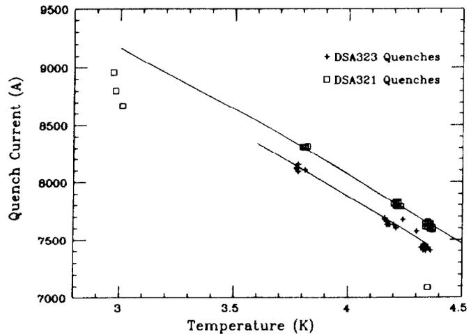
Fig.3: Quench Currents as A Function of Temperature. Solid lines are predictions based on short sample  $I_c$
