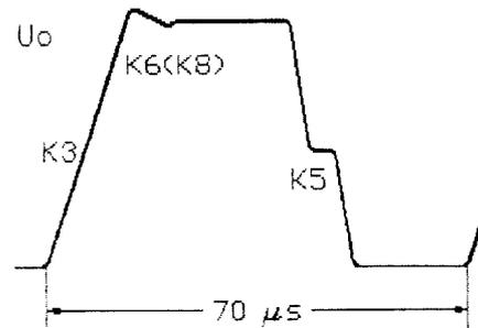
Fig.5 The line voltage
