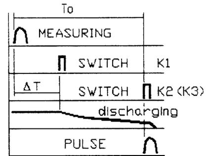
Fig. 2 Time diagram of one turn pulser work
