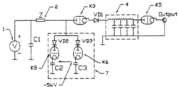
Fig.4 The principle scheme of a multi turn pulser.
