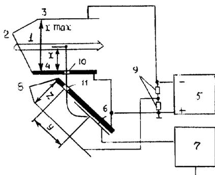
Fig. 1. The circuit of the beam cross section unconnected detector.
