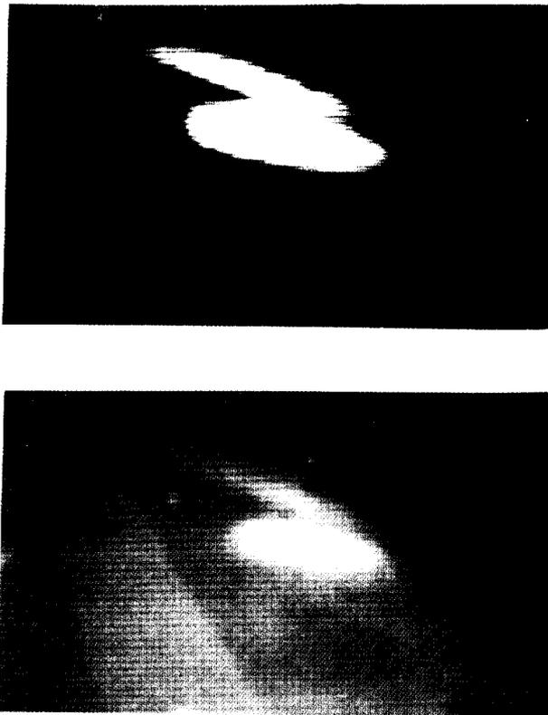
Fig. 2. Picture of the beam transverse cross section from the luminescent screen (a) and unconnected detector EOC screen (b).
