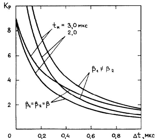
Fig.3. Curves of upgrade factor  $K_p$  v.s. pulse duration  $\Delta t$  for optimum value of coupling factors  $\beta_1$ ,  $\beta_2$  and  $\beta$ .
