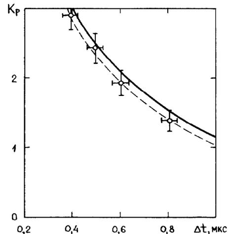
Fig.4. Measured (---) and calculated (—) values of  $K_p$  for cavity with  $Q_0 = 90 \cdot 10^3$  and  $\beta = 10$ .
