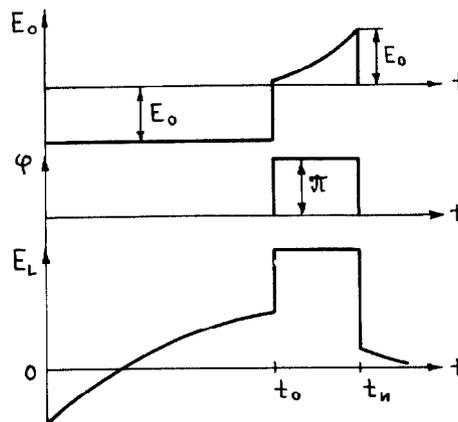
Fig.2. Linac operating time diagrams.
