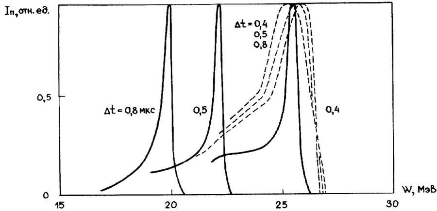
Fig.5. Accelerated beam energy spectra for RF energy compression system with (—) and without (---) amplitude-phase modulation.
