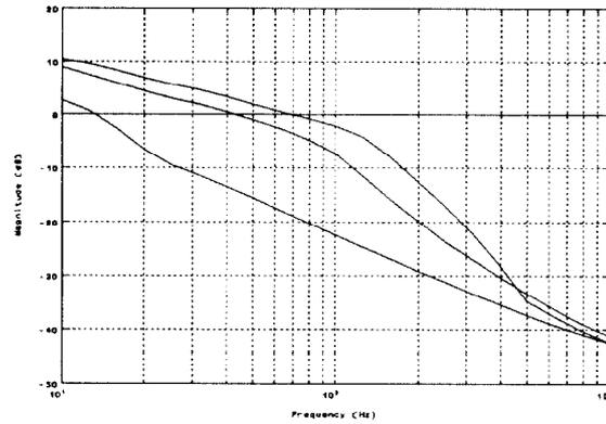
Figure 2 - Magnitude plot of the plant plus the modified bank drive amplifier at different operating points.
