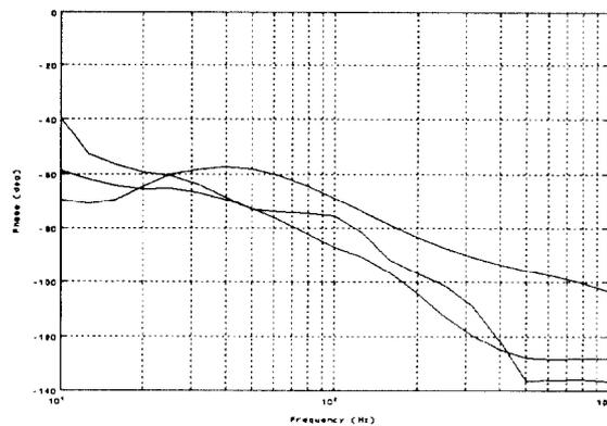
Figure 3 - Phase plot of the plant plus the modified bank drive amplifier at different operating points.
