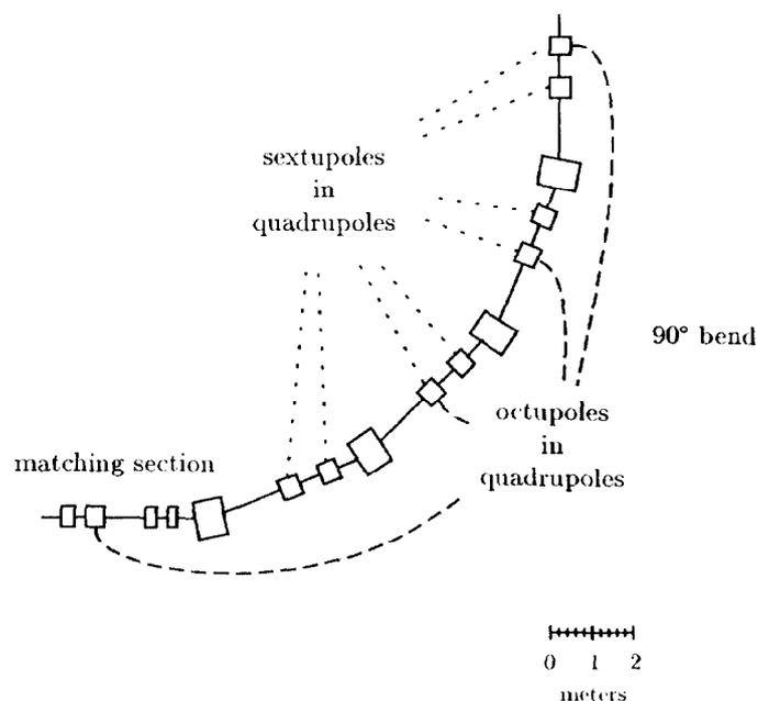
Figure 1. Layout of the PILAC zero-degree injection line.
