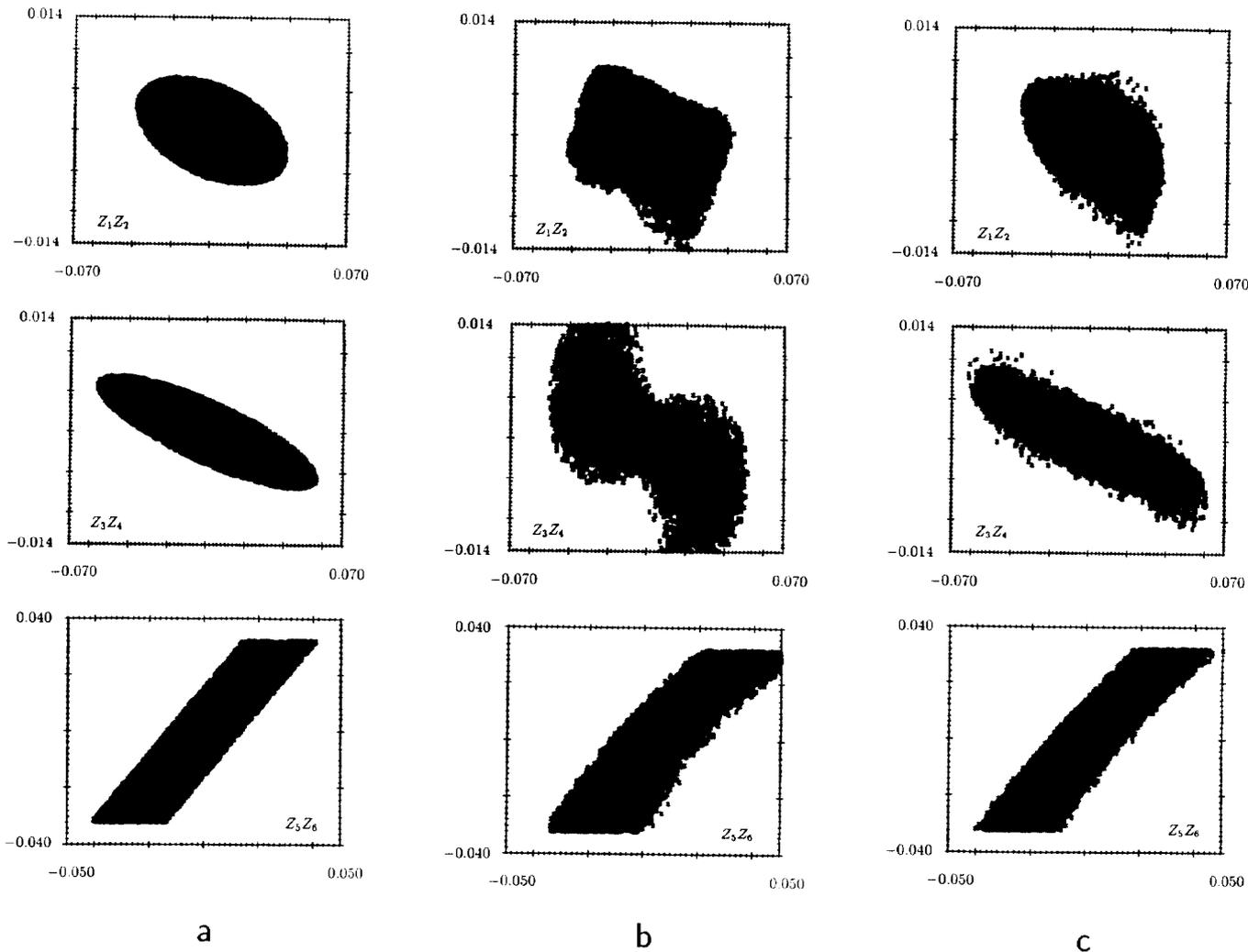
Figure 2. Transverse and longitudinal phase-space projections of the output beam for the injection line (a) in linear approximation, (b) without nonlinear elements, and (c) with nonlinear elements.
