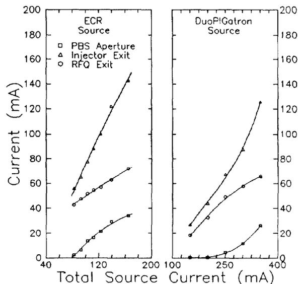
Figure 3. Injection and RFQ output currents for ECR and duoPIGatron ion sources.
