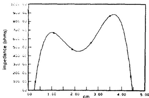
Fig. 3 Interaction impedance for 6-cell TW cavity
