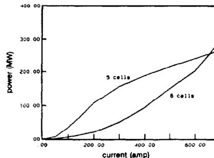
Fig. 6 Comparison of 5- and 6-cell cavity output power
