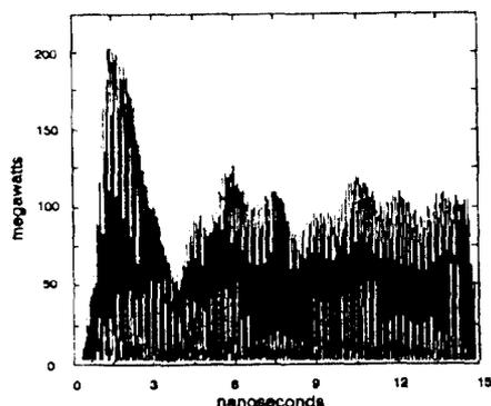
Fig. 5 Output power for a 6-cell cavity
