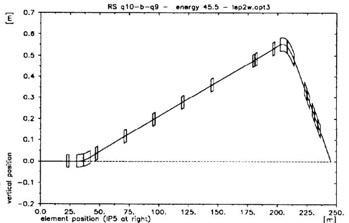
Figure 3: Layout of the Richter-Schwitters spin rotator at IP5 in LEP.
