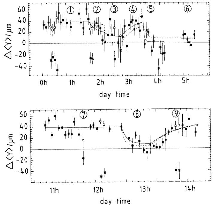
Figure 3: Experimental results in terms of mean shift  $\Delta\langle Y \rangle$  at a beam energy of 46.5 GeV ( $\nu_s = 105.53$ ). Expected behavior from applied depolarizing resonances (dotted line) is compared to the experimental data fit. Negative  $\Delta\langle Y \rangle$  values represent *check measurements* with the push-pull  $\lambda/2$  plate in "IN" position.
