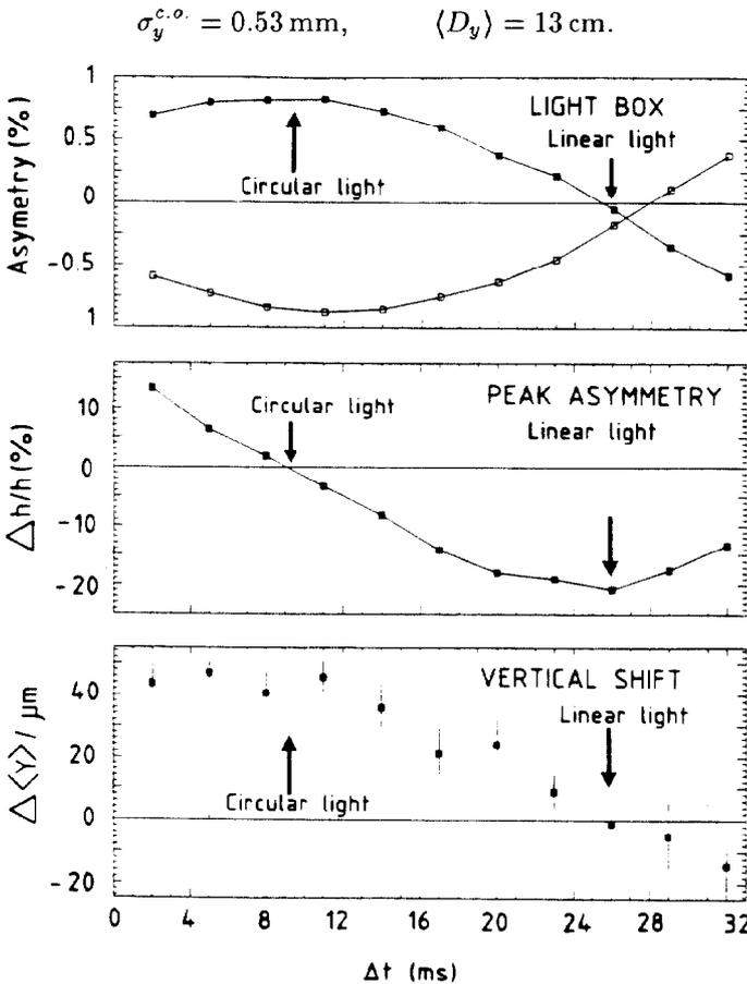
Figure 1: Optimization of the light polarization states.
