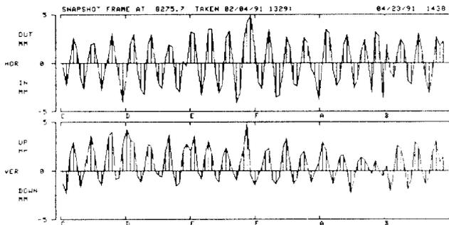
Figure 4: TEVATRON closed orbit at low- $\beta$  with collisions occurring at B0.
