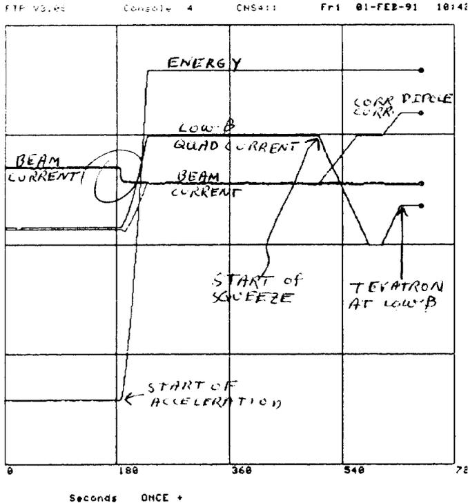
Figure 3: TEVATRON  $p$  intensity during acceleration and squeeze. This plot is taken from the TEVATRON logbook and shows the TEVATRON energy, beam current, one of the low- $\beta$  quadrupole currents, and a correction dipole current.
