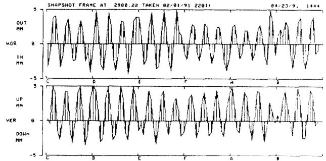
Figure 2: 150 GeV closed orbit with separators on.
