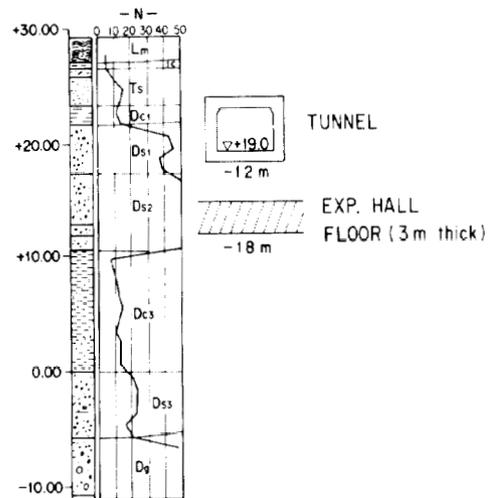
Fig.2 Typical underground N-value variation of the KEK site.
