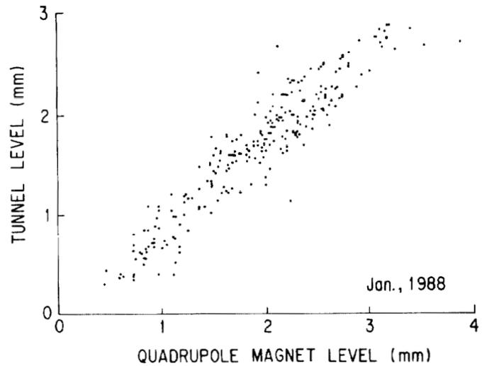
Fig.3 Correlation of levels between quadrupole magnets and fiducial points ( measured at Jan. 1988).
