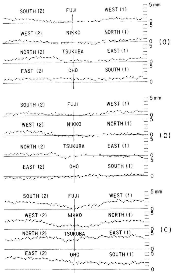
Fig.4 Relative level variations of the MR quadrupole magnets, (a) Oct. 1986 (b) May, 1987 (c) Jan. 1988.
