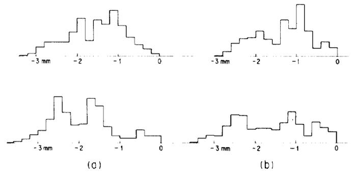
Fig.5 Distributions of magnitudes of level change for (a) quadrupole magnets and (b) tunnel floor. Upper: May, 1987, Lower: Jan., 1988. Horizontal scale is only for reference.
