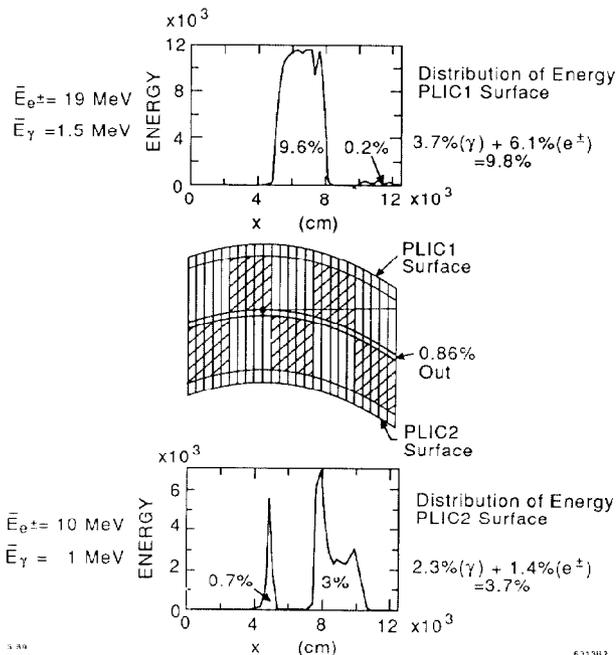
Fig. 1: Energy reaching PLIC surfaces in SLC Arcs.
