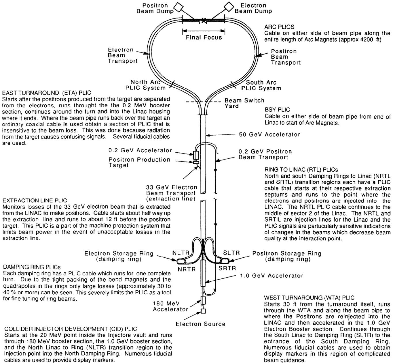
Fig. 3: Overall SLC layout, showing PLIC installations.
