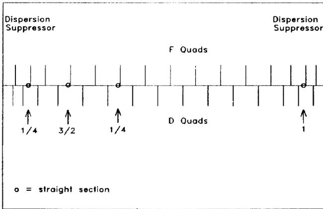
Figure 4: Schematic layout of lattice for Option 3. The circles indicate the medium (3/2), mini (1), and *micro* (1/4) straight sections.
