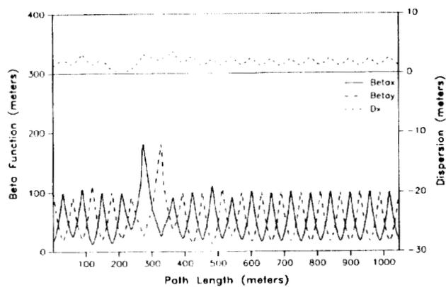
Figure 3: Normal superperiod for Upgrade lattice - Option 2
