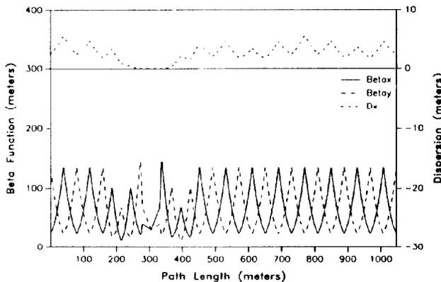
Figure 5: Normal superperiod for Upgrade lattice - Option 3
