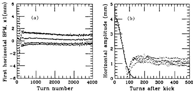
Figure 2. Typical data from the E778 experiment, showing both Gaussian decoherence and a persistent signal.
