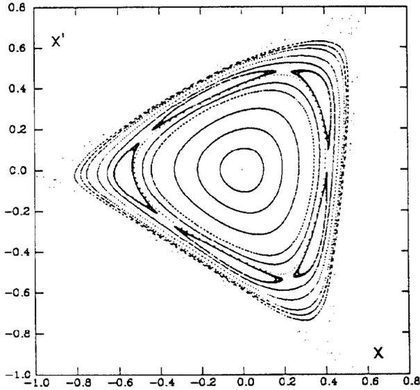
Figure 1. Surface of section plot from a simulation of E778, with islands at an amplitude of about 5 mm ( $\beta \approx 100$  meters).
