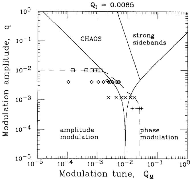
Figure 3. The four dynamical phases in the tune modulation parameter space  $(Q_M, q)$ , for a typical  $Q_I = 0.0085$ . The region accessible to the E778 experiment is shown by the dashed line.
