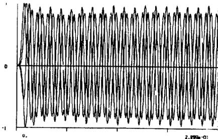
Fig. 4 SL4 cavity 3 quadrupole wakes for 0.3 meters.
