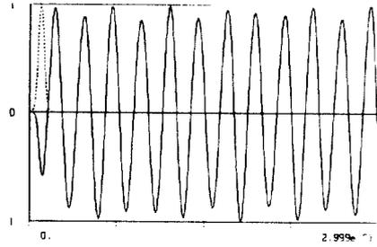
Fig. 5 SL4 cavity 5 monopulse wake for 0.3 meters.
