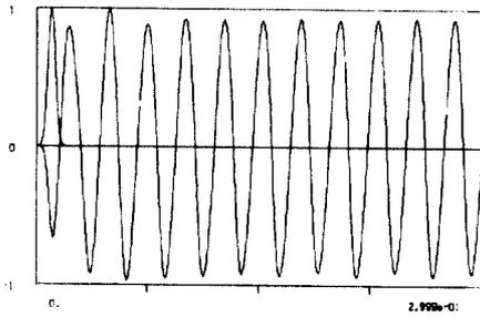
Fig. 2 SL4 cavity 3 monopulse wake for 0.3 meters.
