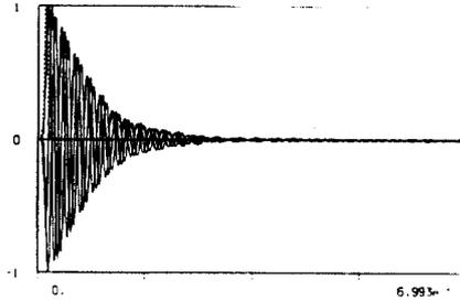
Fig. 3 SL4 cavity 3 dipole wakes for 0.7 meters using a 70 cm beam pipe.
