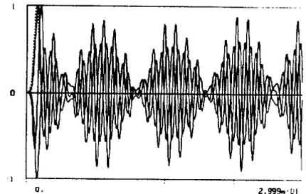
Fig. 7 SL4 cavity 5 quadrupole wakes for 0.3 meters.
