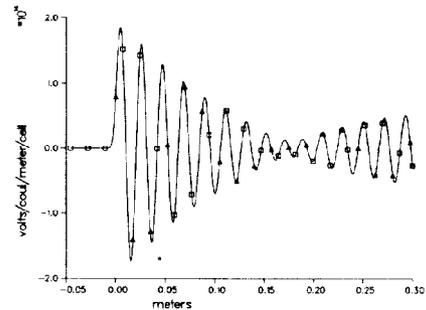
Fig. 9 Transverse dipole wakes from TBCI and AMOS for 0.3 meters for pipe length = 7.46 cm.
