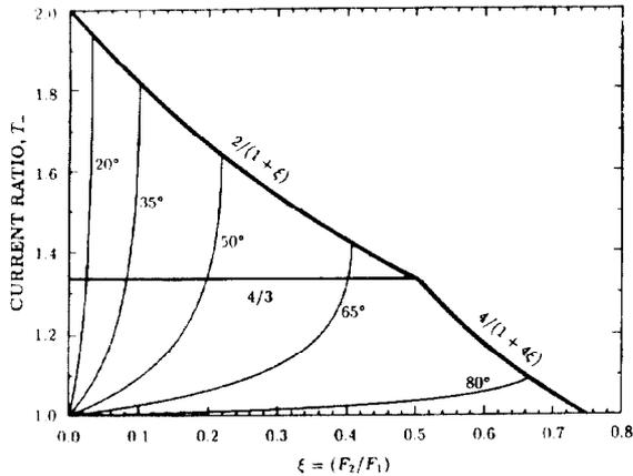
Fig. 3. The current ratio  $T_-$  as a function of  $\xi$  for various values of the detuning angle  $\phi_y$ . Thick curves correspond to the extreme values of  $T_-$ .
