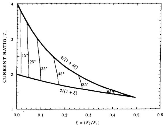
Fig. 4. The current ratio  $T_+$  as a function of  $\xi$  for various values of the detuning angle  $\phi_y$ . Thick curves correspond to the extreme values of  $T_+$ .
