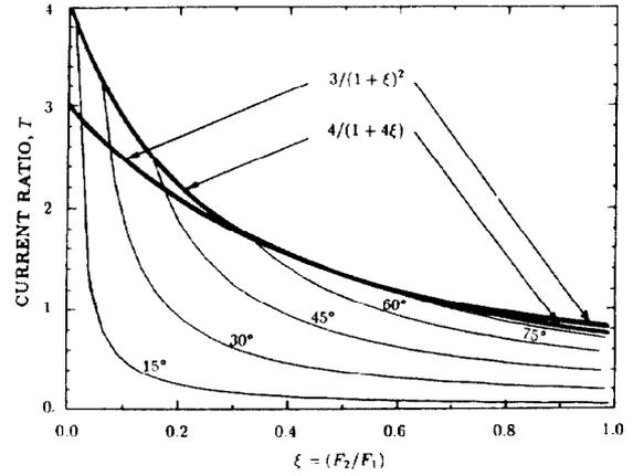
Fig. 5. The current ratio  $T$  as a function of  $\xi$  for various values of the detuning angle  $\phi_y$ . Thick curves correspond to the extreme values of  $T$ .
