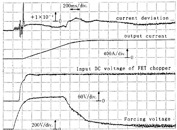
Fig.6 Waveform of bending magnet power supply
