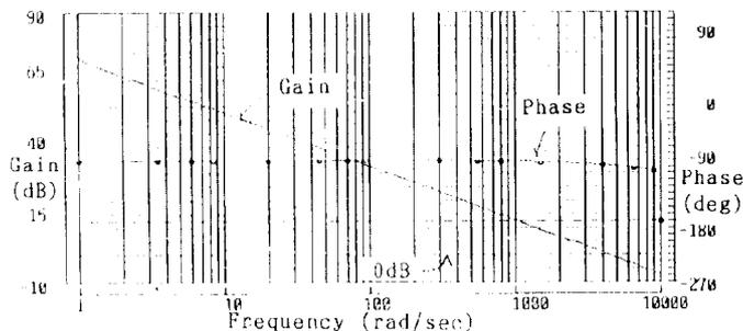
Fig.3 Bode diagram of ACR of bending magnet power supply
