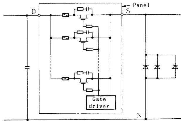
Fig.5 Circuit diagram of FET panel
