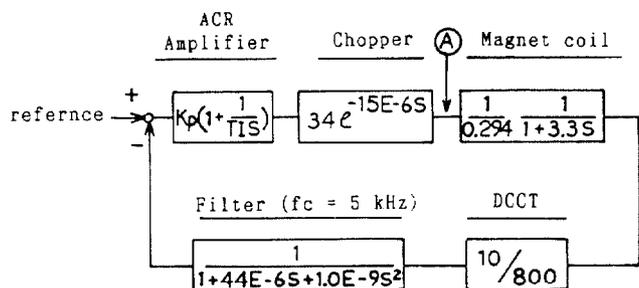
Fig.2 Block diagram of ACR of bending magnet power supply
