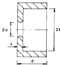
Figure 2 - Geometrical parameters of the accelerating cell.
