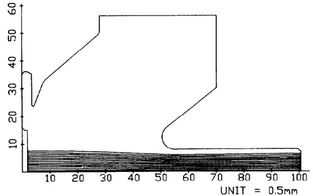
Figure 4 - Electron trajectories.
