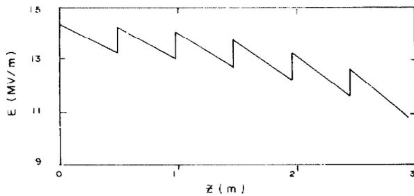
Figure 3 - Accelerating gradient along one structure
