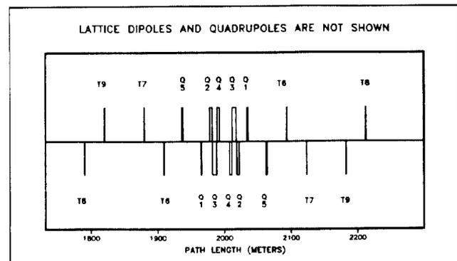
Figure 1. Elements of the low  $\beta$  lattice.
