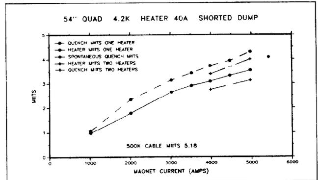
Figure 5. Quench protection-heater induced Miits.
