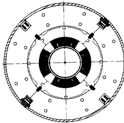
Figure 2. Cross-section of the two-shell quadrupole.
