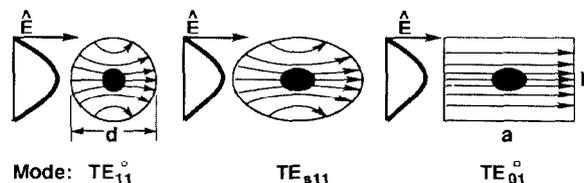
Figure 1. Commonly-used IW cross sections, modes, and optical E-field intensity.
