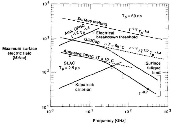
Figure 2. Electrical breakdown and metal fatigue limits on surface electric field for copper.
