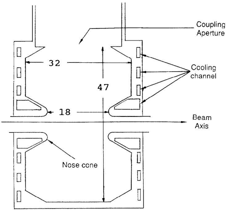
Figure 2. Cross section of MCTD cavity showing important dimensions (cm).
