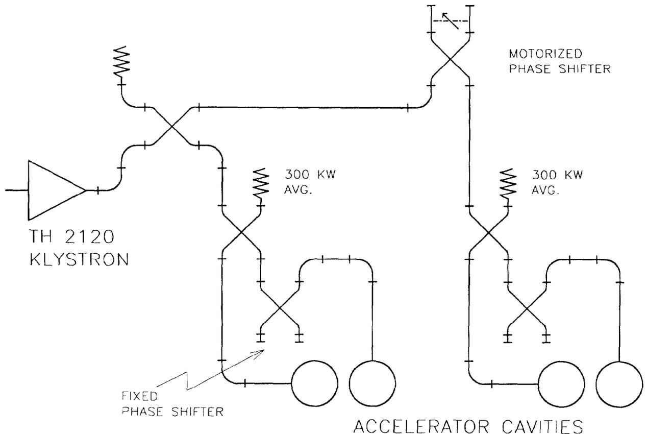
Figure 1. Schematic of RF feed system for MCTD accelerator module.
