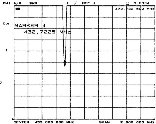
Figure 3. Network analyzer traces for finished MCTD cavity, from which a coupling coefficient of 5.6 and  $Q_0$  of 40,000 can be determined.
