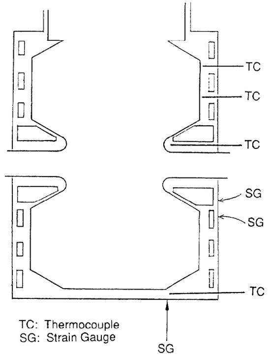
Figure 4. Deployment of some of the thermocouples and strain gauges to be used in MCTD cavity high power test.
