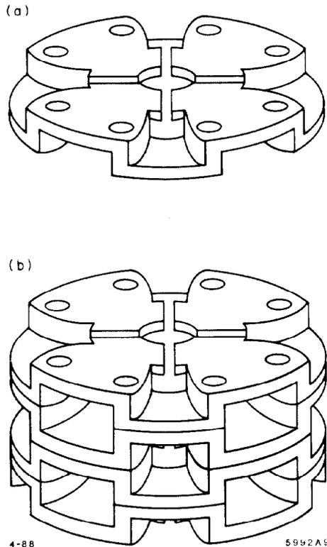
Fig. 1. Accelerator structure with  $HEM_{11}$ -mode damping.
