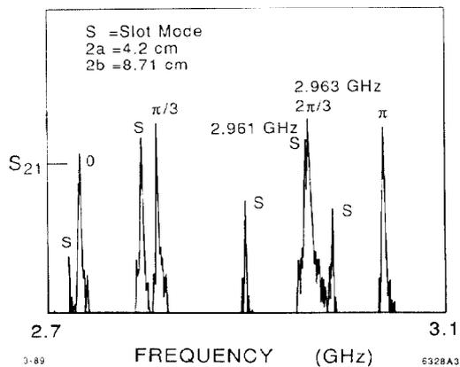
Fig. 3.  $S_{21}$  Plot: Large beam aperture, slots aligned.
