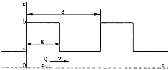
Fig. 1 Periodic structure repeating the gap g with a period d.
