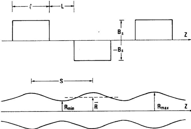
Fig. 2. Schematic of periodic focusing field and matched beam.
