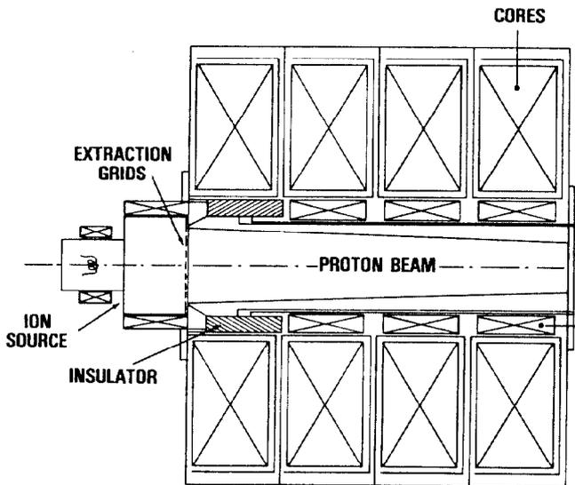
Fig. 1. Schematic of ion source and preaccelerator.
