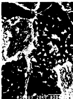
Fig. 5 Scanning electron micrography of the pyramid population appearing in the ferrite region of the bombarded surface
