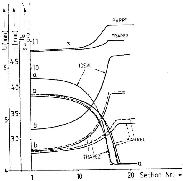
Fig. 4 Slopes of geometric data vs.  $\beta\lambda$  cell number with  $\beta = 0.4$ , variable  $s$  ----, fixed  $s$  ———. Note that both profiles answer the purpose of acceleration from 10 - 300 keV along a distance of about 42 cm with 21 kV electrode voltage, while ideal electrodes need 25 kV.
