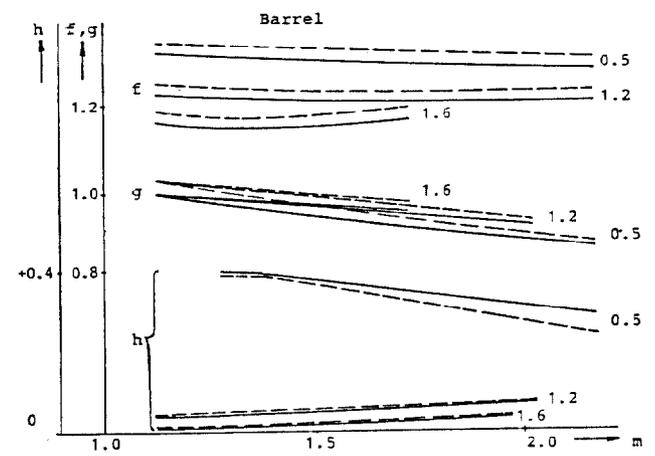
Fig. 2 Correction factors vs. modulation for different parameters  $ka$ ,
