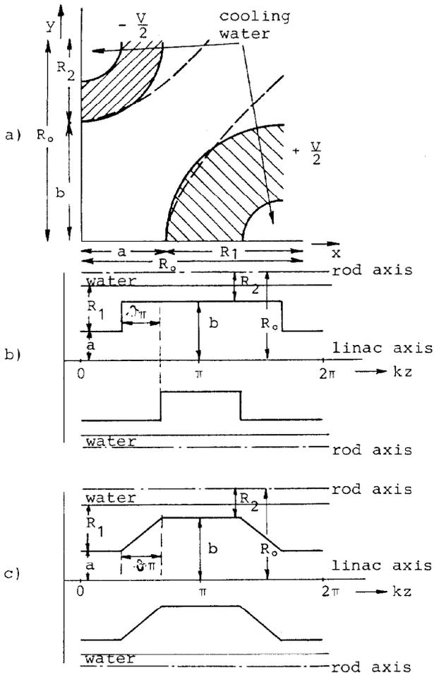
Fig. 1 Cross sections of RFQ rods
