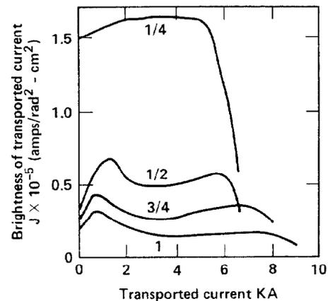
Fig. 8. Computer simulations on how beam brightness is improved, at the cost of transported beam current, by lowering the magnetic field that is used for total peak current transport.
