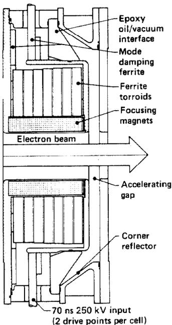
Fig. 1. Cutaway view of the components inside one accelerating case.
