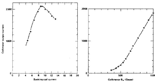
Fig. 7b. (Left) Varying the magnetic flux on the cathode surface by using a Bucking Coil changes the effective total beam emittance by canceling beam angular momentum. Figure 7c. (Right) Varying the  $B_z$  field over the solenoid/ collimator controls the output current in a manner that suggest non-uniform phase space distributions (nonlinear  $\alpha$ ).
