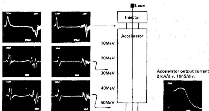
Fig. 4. With laser guiding transport of the beam through the accelerator, there is minimal BBU growth and pulse disruption.
