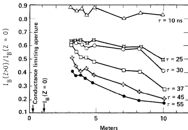
Fig. 5. Vacuum expansion of the electron beam as it exits the ion column and free transports into a six inch diameter pipe indicates that beam angles increase during the pulse, an observation consistent with intrapulse ionization of the benzene.
