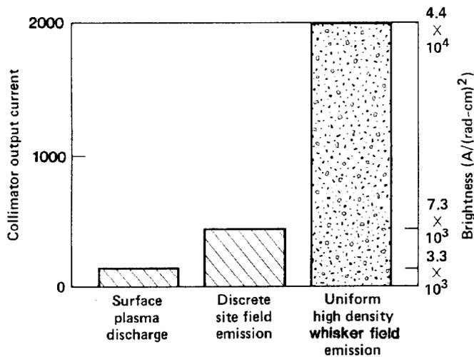
Fig. 7a. For various cathode surfaces that have been tested, the current through a  $B_z$  immersed collimator indicates the emittance and brightness.
