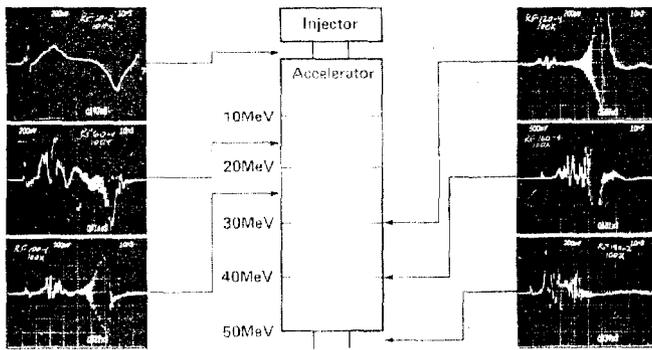
Fig. 2a. Magnetic induction signals indicating growth of BBU transverse motion as the beam transports through the ATA when using customary magnetic transport.
