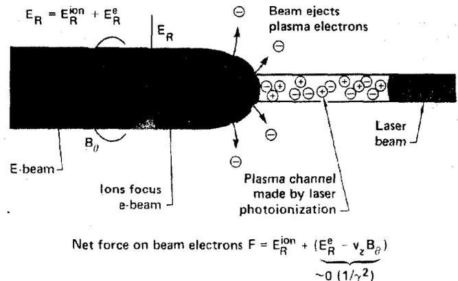
Fig. 3. The essence of laser guiding is that a laser preionizes a small diameter plasma column and that when the relativistic beam is injected onto this column the secondary electrons are expelled having a strongly focusing, positive ion column.
