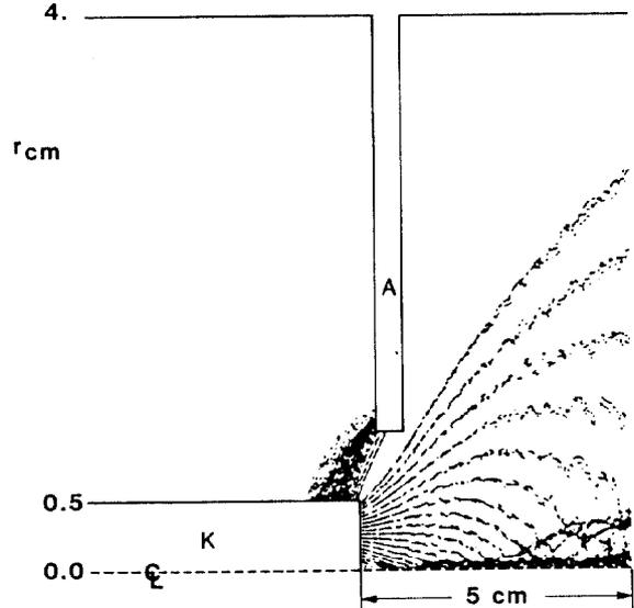
Figure 5. Electron map from MAGIC simulation at  $t = 2.4$  ns for a 1-MeV diode with  $n_c = 8 \times 10^{11} \text{ cm}^{-3}$ . Total current was 19 kA, with 5 kA transported on axis.
