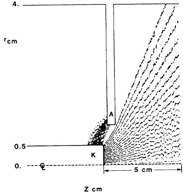
Figure 4: Electron map from MAGIC simulation at  $t = 3.2$  ns for a 1-MeV diode with  $n_c = 0$ . Total current was 18 kA, with 3 kA transported on axis.
