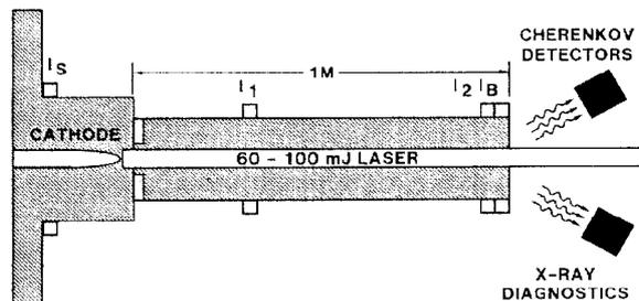
Figure 1: Schematic of laser diode and transport experiment.
