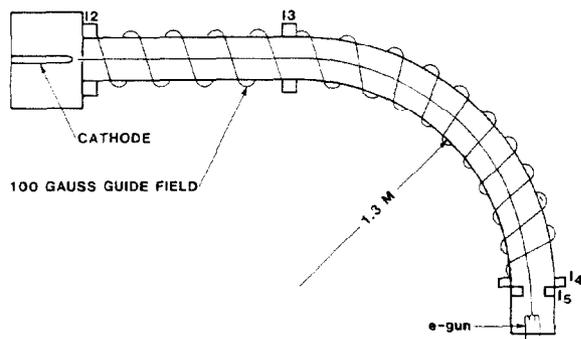
Figure 7: Schematic of 90° bending experiment.
