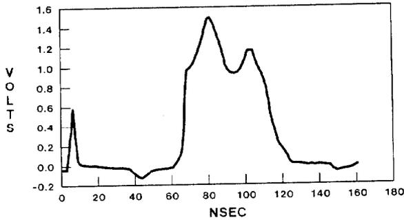
Figure 3: Cherenkov photodiode output. The fast risetime is due to the 300 KeV threshold
