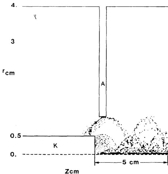
Figure 6: Electron map from MAGIC simulation at  $t = 2$  ns for a 1-MeV diode with  $n_c = 8 \times 10^{12}$   $\text{cm}^{-3}$ . Total current was 21 kA with 15 kA transported on axis.
