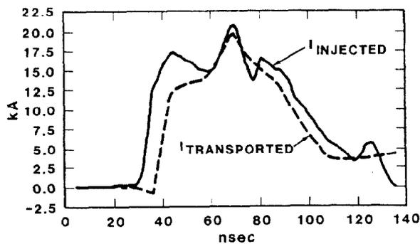
Figure 8: Current transport efficiency around a 90° bend of a 1-MeV beam in 1 mTorr of argon.
