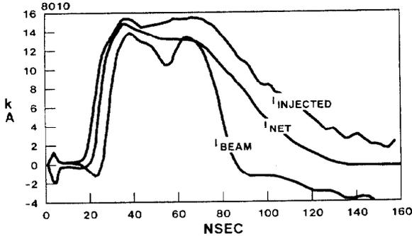
Figure 2. Current transport showing the injected net current and the transported net and beam current of a 1-MeV beam in .3 mTorr of DEA.
