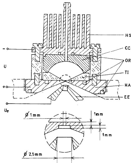
Fig. 2. Cross-sectional view of the hollow anode ion-electron source: HS - heat sink, CC - concave cathode, OR - "O" rings, TI - teflon insulator, HA - hollow anode, EE - extraction electrode, U - discharge voltage, and  $U_e$  - extraction voltage.
