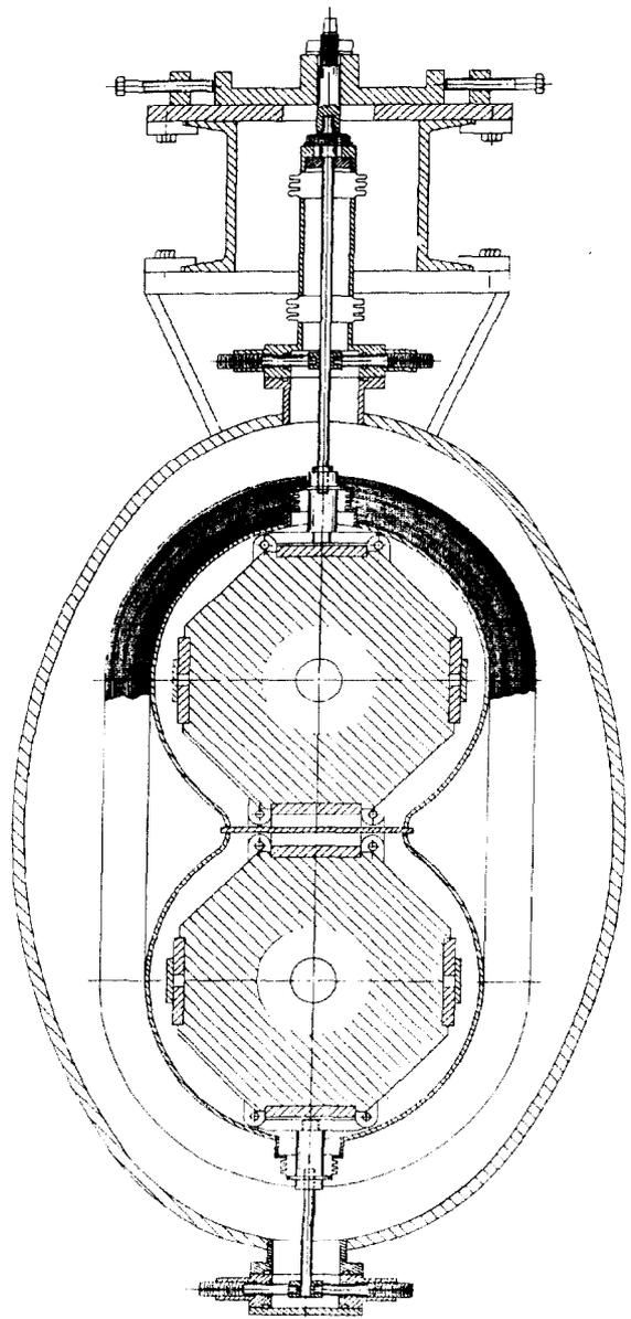
Fig. 2 Cross Section of Magnet Dewar
