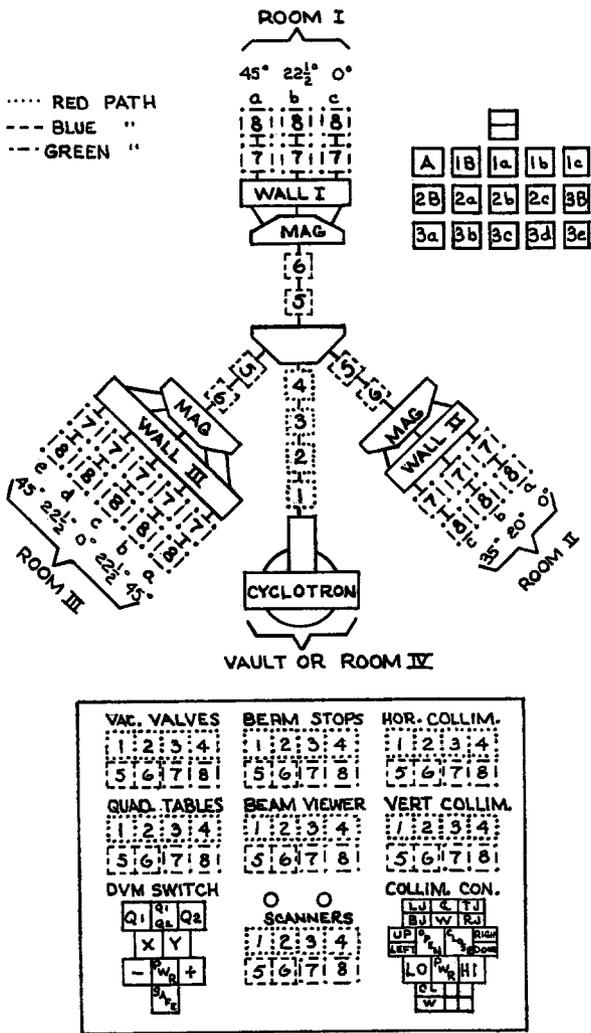
Figure 2 - The Path Display and Control Panel
