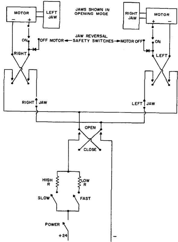
Figure 6 - The Collimator Control Circuit
