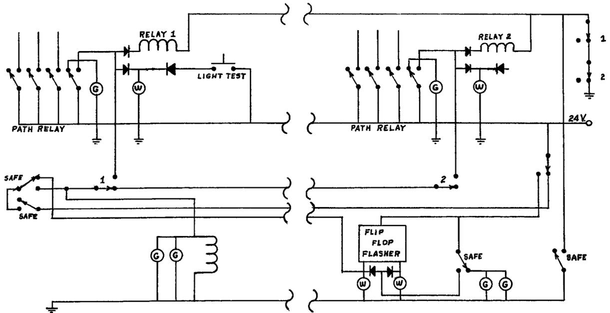
Figure 3 - The Path Selection Circuit
