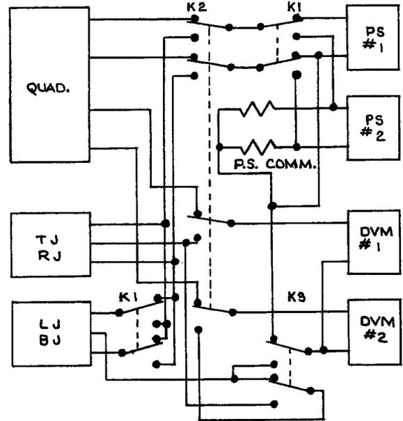
Figure 7 - The Voltmeter and Power Supply Programming Circuit
