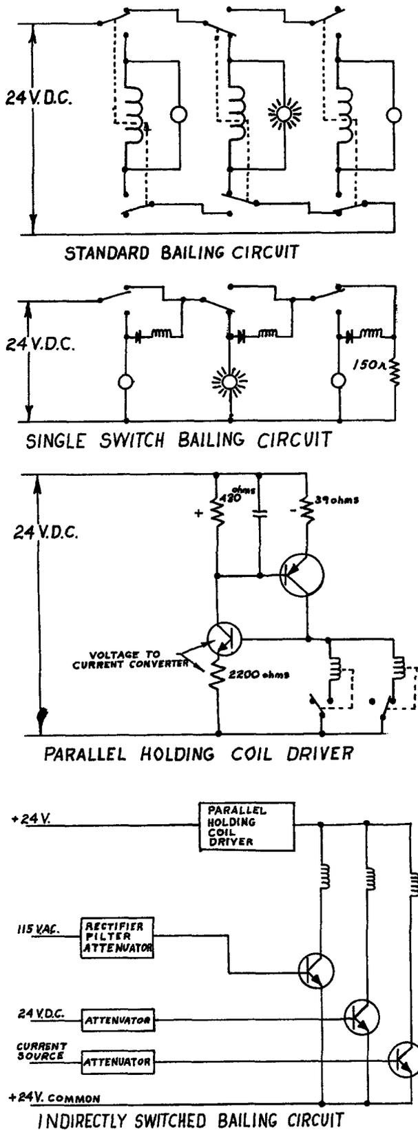
Figure 5 - The Switch Bailing Circuits
