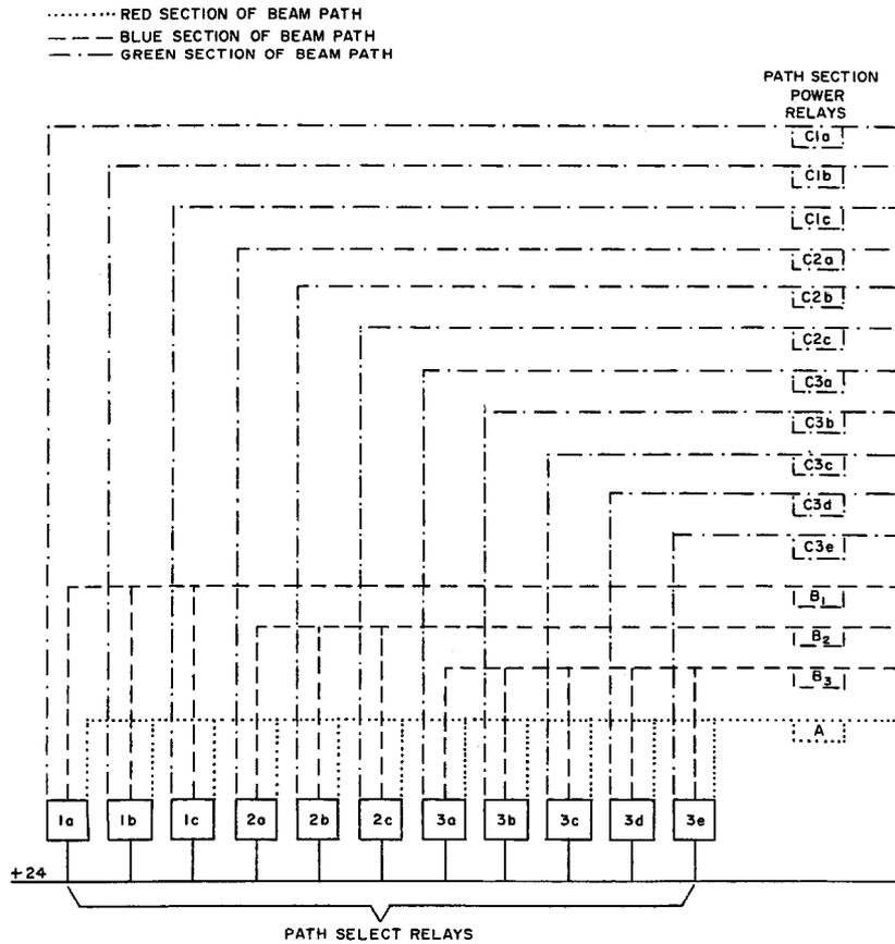
Figure 4 - The Path Relay Matrix
