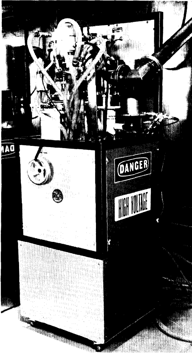
Fig. 7. Photograph of 350 kW driver amplifier cart.
