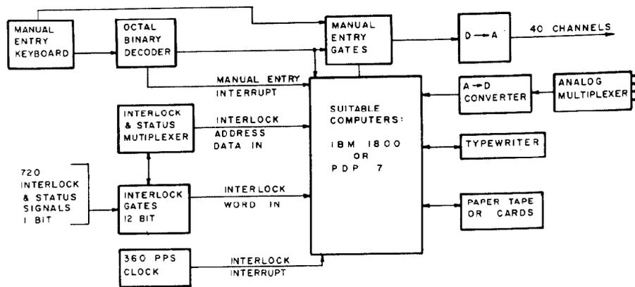
Fig. 4. Control computer system.
