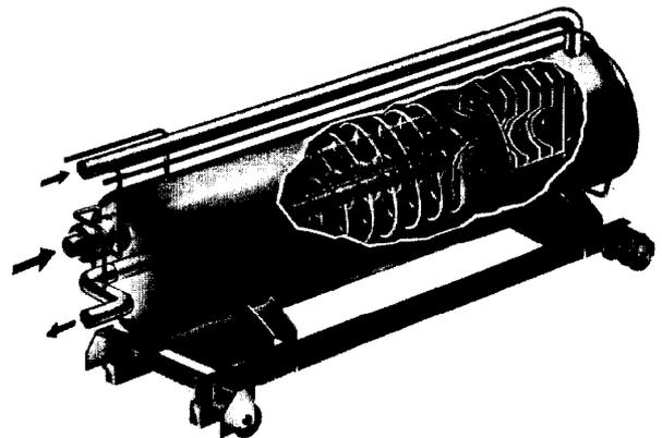
Fig. 2. 2.2 MW beam dump.
