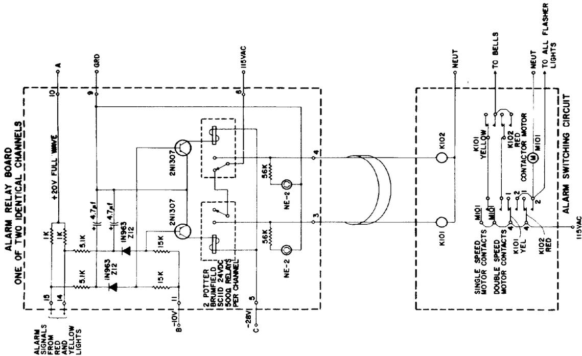
Fig. 4 Neutron System Alarm Circuit.
