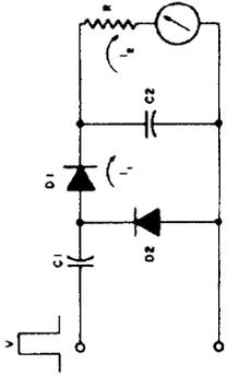
Fig. 5 Neutron System Diode Pump Circuit.
