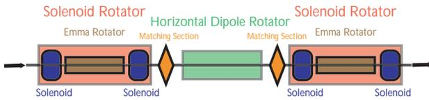
Figure 1: The ILC Spin Rotator schematic.
