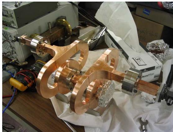
Figure 7. The assembled X-band alumina based gapless DLA structure.
