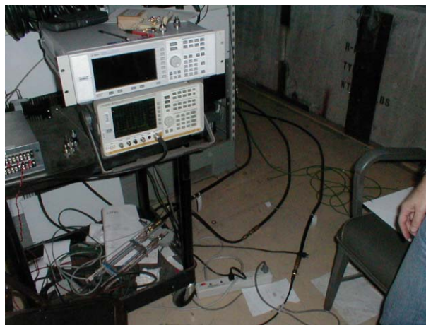
Figure 3: Instruments setup in the IR12 experimental hall. The RF cables from the BPM are visible on the floor.
