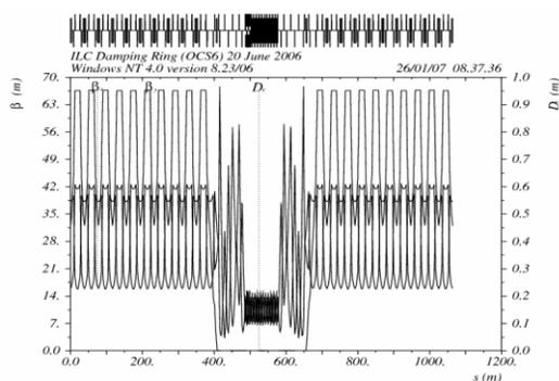
Figure 1: Twiss parameters of 1/6 section in the OCS6 damping ring that is used in the simulations.
