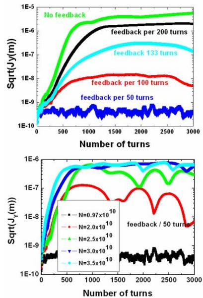
Figure 4: (Top) Vertical amplitudes for the different number of the feedbacks in the case A. (Bottom) Vertical amplitudes for the different bunch intensities with the feedback per 50 turns in Case A.
