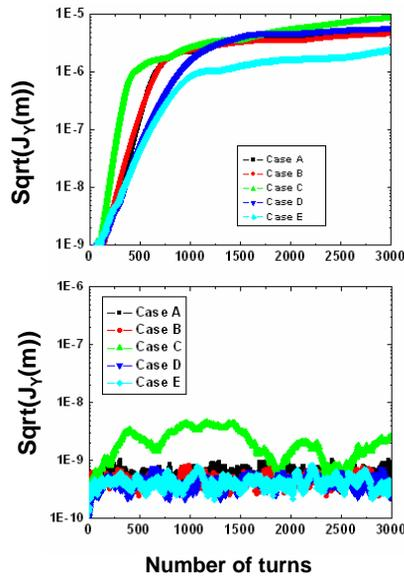
Figure 2: Vertical amplitudes for the five filling patterns without the feedback (top) and with the feedback per 50 turns (bottom). Case A, B, C, D and E show the exponential growth times of 84, 96, 67, 143 and 213 turns, respectively.
