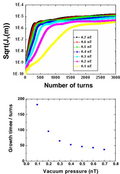
Figure 3: (Top) Vertical amplitudes for the different vacuum pressures in Case A. (Bottom) shows the exponential growth times in the different vacuum pressures.
